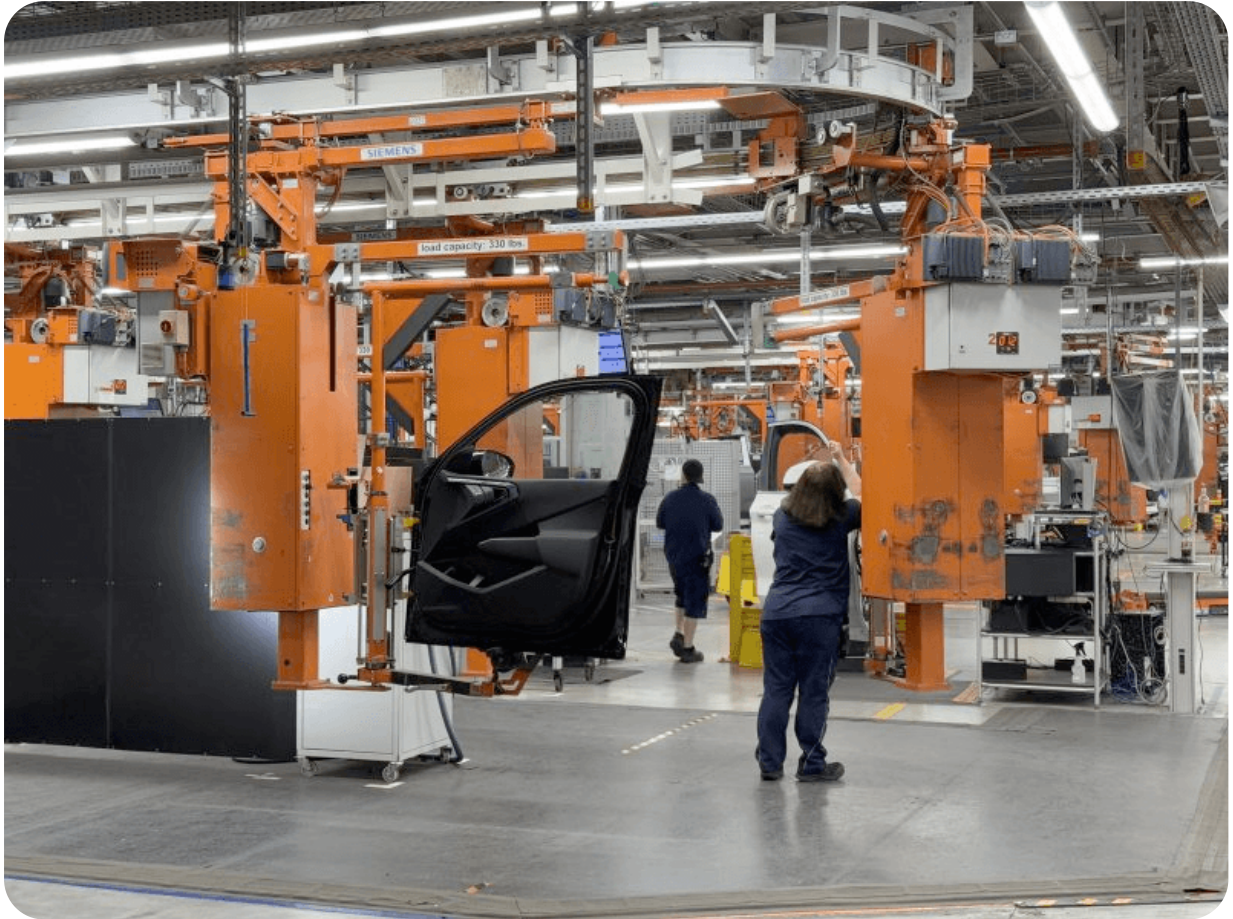
Production line with car doors, which are currently manually inspected after assembly
